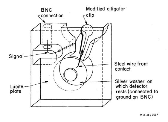
Fig. 6. Diagram of counter holder.
