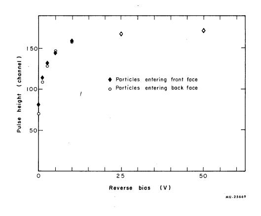
Fig. 5. Pulse height vs bias voltage.
