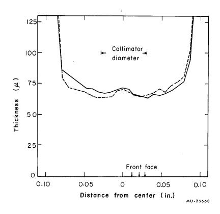
Fig. 3. Typical thickness profile after etching. Two sections at right angles are shown.
