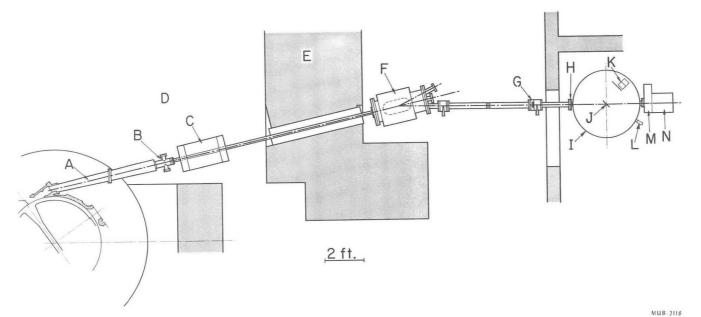
Fig. 1. Experimental arrangement: A, iron pipe; B, adjustable slit; C, quadrupole focusing magnet; D, cyclotron vault; E, shielding wall; F, steering magnet; G, 3/16-in.-diameter graphite collimator; H, 3/16-in.-diameter tantalum baffle collimator; I, 36-in. scattering chamber; J, target; K, counter telescope and foil wheel; L, monitor; M, foil wheel for measuring beam energy; and N, Faraday cup.
