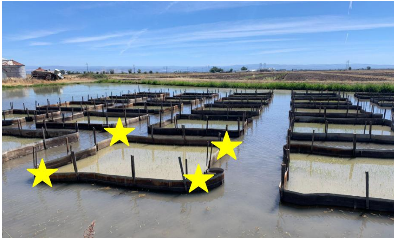
Figure 25: Photo of field layout of fish density experiments. Stars indicate sampling location within each ring. Trials A and B sampled bottom left and top right corners only. Trials C and D sampled all four corners.
