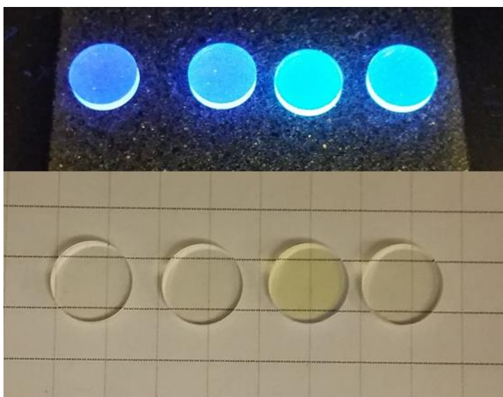
Figure 38 – Wavelength shifter test samples under UV(Top) and room (Bottom) lighting. The samples contain (from left to right) TFS, Coumarin 500, ADS086BE, and ADS129BE. The samples show excellent transparency.
