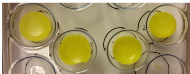
Figure 32 – Samples seen in Figure 31 after demolding and removal of foaming. TFS concentration increases from left to
