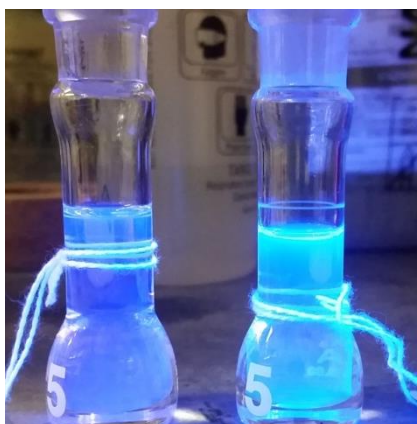
Figure 36 - DMT-DCz exhibits clear solvatochromism. Under UV light, the color difference from solutions in Toluene (left) to Chloroform (right) is visible to the naked eye.
