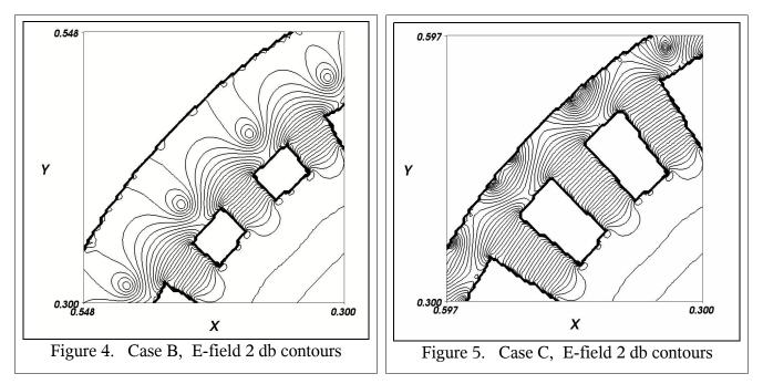
Figures 4 and 5 show the results for the electric field magnitude for cases B and C with similar results and agreement with the waveguide-beyond-cutoff model.
