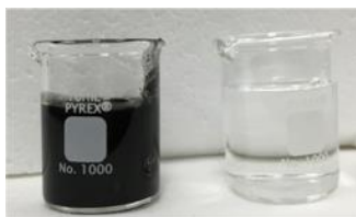
Figure 5: Raw fracking samples (left) compared to ultrapure (>18 MΩ/cm) water (right).
