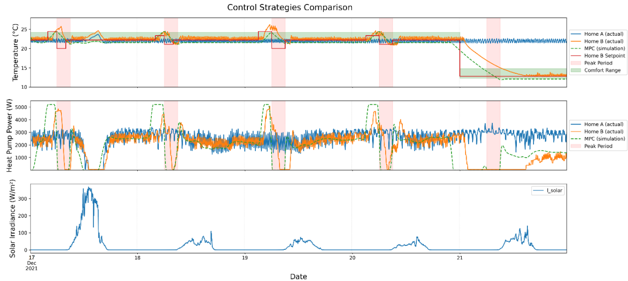
Figure 10. MPC simulation results and the comparison with real measurements. Top: setpoint and indoor temperature in lines, comfort range in green horizontal bands, peak hours in red vertical bands; Middle: heat pump power demand in lines, peak periods in red vertical bands; Bottom: solar irradiance
