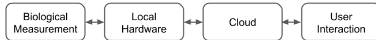
Figure 1.1: Cloud-based experiment paradigm. Biological measurement and local hardware are presented to the user through the cloud, such that experiment management and control can be administrated remotely and may be automated by a computer program.
