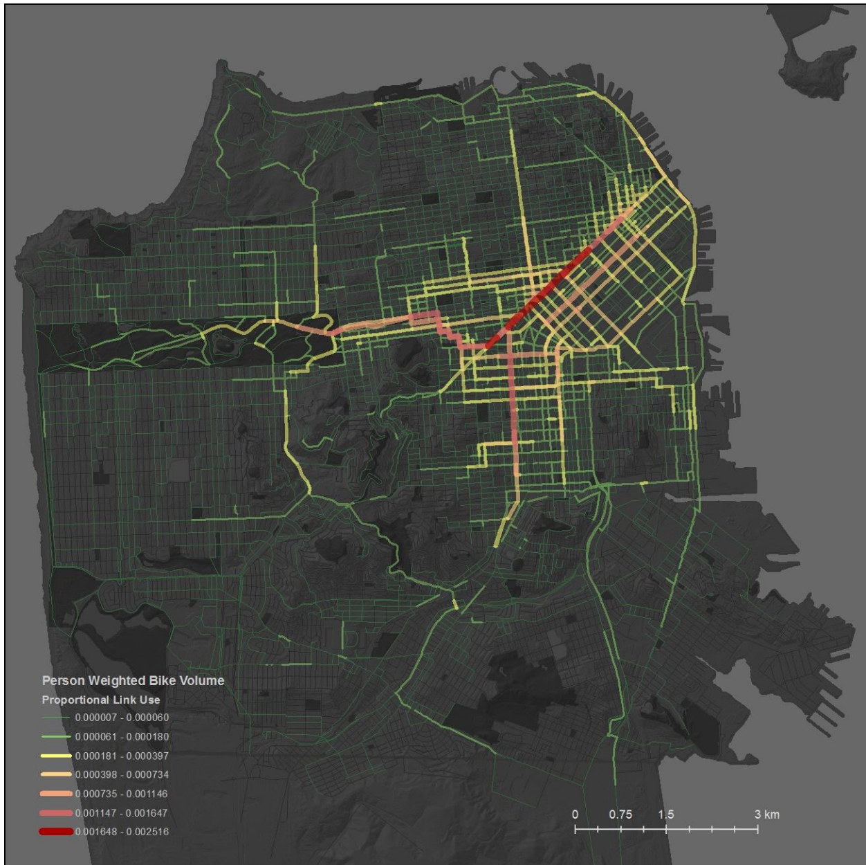
Figure 3.3 Weighted bike volume as proportion of network link use. Reprinted from "Bicyclist behavior in San Francisco: a before-and-after study of the impact of infrastructure investments," by Fitch et al. (2016a). National Center for Sustainable Transportation Research Report.
