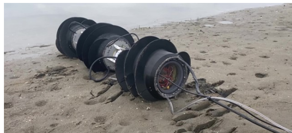
Figure 3.6: ARCSnake V2 demonstrated swimming capability even with only two screws spinning (left). However, due to motor issues the screw shells could not be driven strong enough to screw through the wet compact sand (right).
