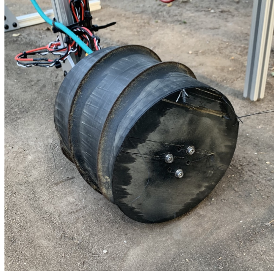
Figure 2.5: During the load experiments, in sand (left) the screw quickly dug itself deeply into the material, and in dirt (right), the screw dug itself into a rock bed, both of which caused slippage on the linear axis motor leading into inconsistent velocity readings. Therefore a lower axial load of 6N instead of 12N was used for these media.
