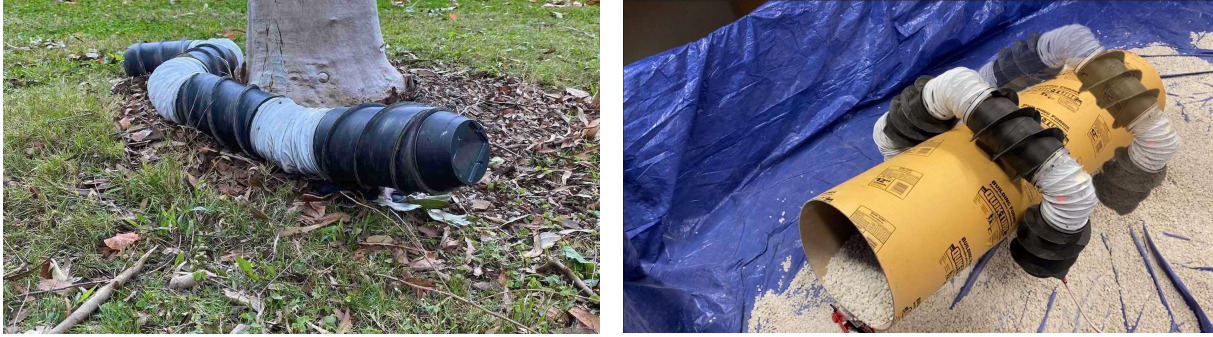
Figure 1.1: ARCSnake V1 showcases the multi-domain ability of a screw-propelled snake robot, which can even grip and climb a pole (right).
