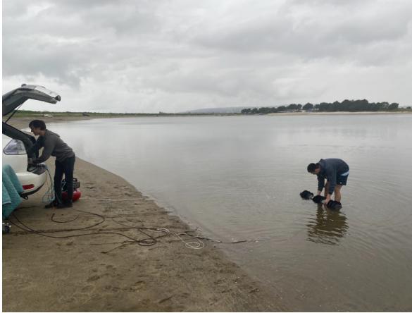
Figure 3.5: Testing ARCSnake V2 at Mission Bay, San Diego. The robot is tethered to a desktop computer, power supply, and air compressor (right).
