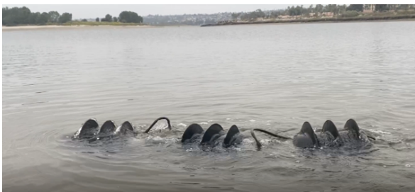
Figure 3.6: ARCSnake V2 demonstrated swimming capability even with only two screws spinning (left). However, due to motor issues the screw shells could not be driven strong enough to screw through the wet compact sand (right).
