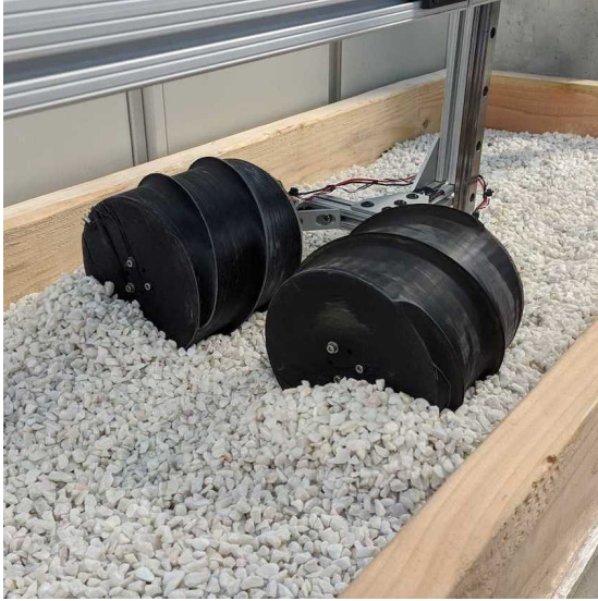
Figure 2.8: Figures from the parallel configuration experiments where the media is small gravel and small gravel & sand as shown in the left and right figures, respectively.
