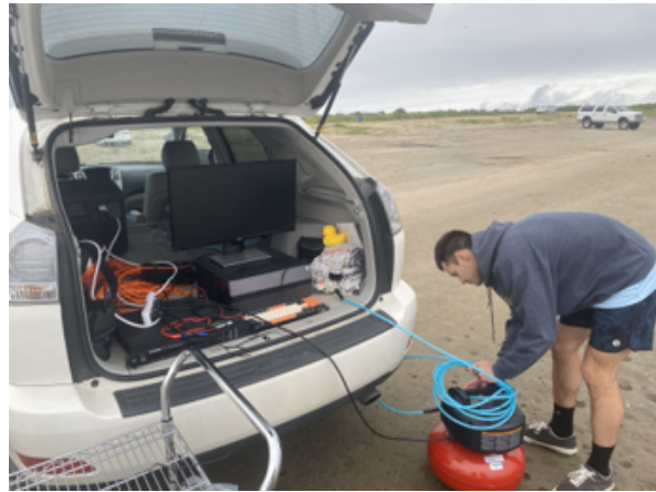
Figure 3.5: Testing ARCSnake V2 at Mission Bay, San Diego. The robot is tethered to a desktop computer, power supply, and air compressor (right).
