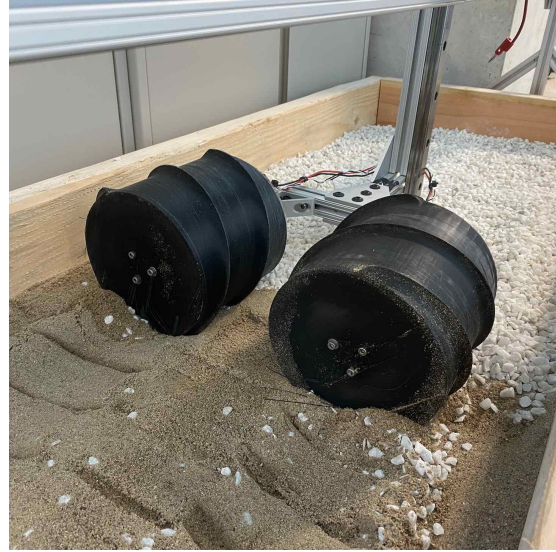
Figure 2.8: Figures from the parallel configuration experiments where the media is small gravel and small gravel & sand as shown in the left and right figures, respectively.
