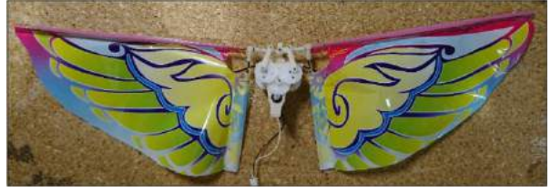
(b) Modified version of the Flapping Wing Air Vehicle with an active mechanism (top view)
