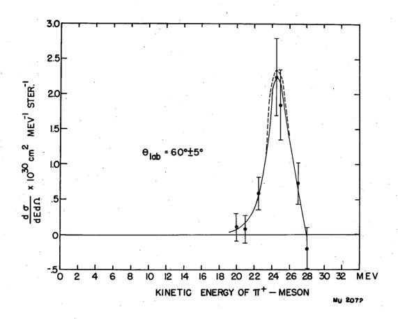
Fig. 1  $\text{Spectrum of } \pi^+\text{-Mesons at } 9 = 60^\circ \pm 5^\circ$  to the Proton Beam
