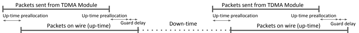
Figure 3.3: A TDMA schedule. Up-time preallocation and guard time correct for observed delays and variance in packet transmission from NIC hardware.
