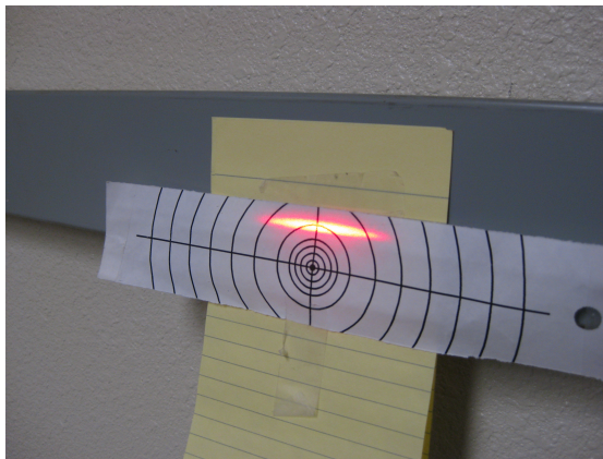
Figure 9.13: A centered beam on the wall target after adjusting central table position
