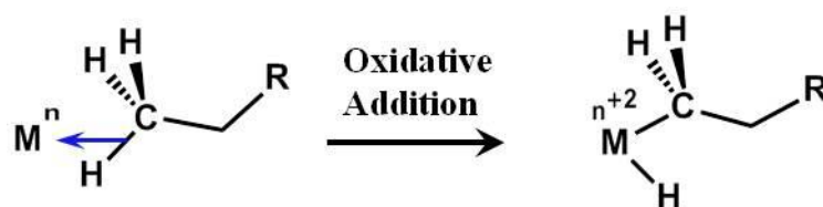
Scheme 3.1. Formation of a \eta^2 -H,C alkane \sigma -complex prior to oxidative addition.
