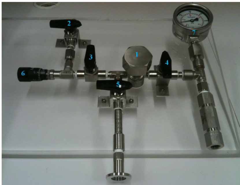
Figure 3. 28. Image of the pressure cell used for the SC–SC transformation experiments with argon and xenon gas. Goniometer pin is placed underneath cap labeled (1), further details in Section 3.19.
