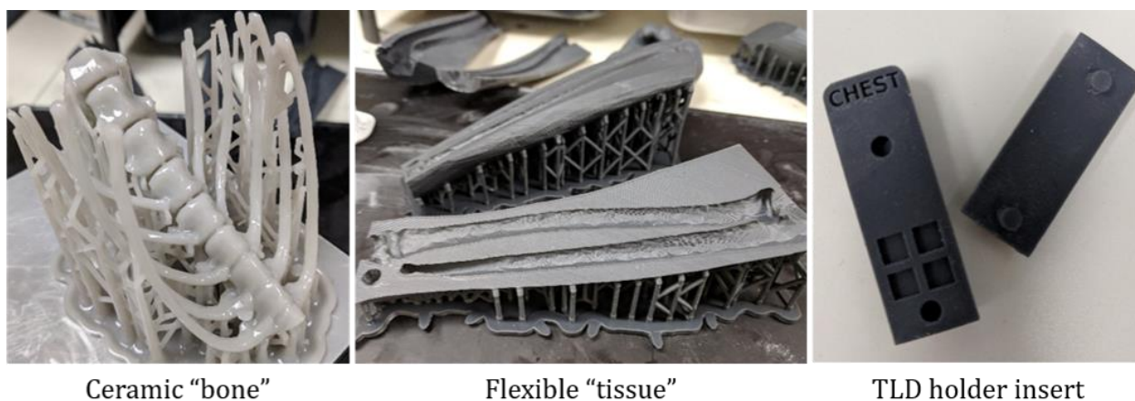
Figure 3-9 3D printed monkey phantom parts. The bone segments were printed out of Ceramic Resin (left) and soft tissue out of Flexible Resin (center). Inserts in the phantom abdomen and chest were designed for TLD dosimetry (right).
