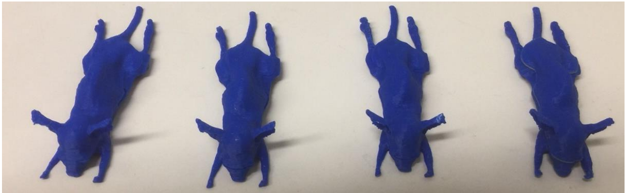
Figure 3-3 Phantoms 3D printed out of ABS from the CAD model shown in Figure 3-2. The weight of the phantom is 24.5 \pm 0.1 g.
