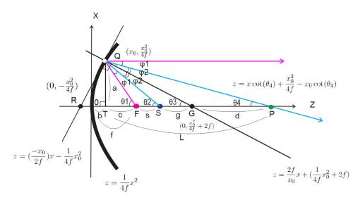
Figure 5.4: Schematics of spherical off focus illumination
