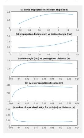
Figure 5.6: Position-dependent conic angle and associated parameters
