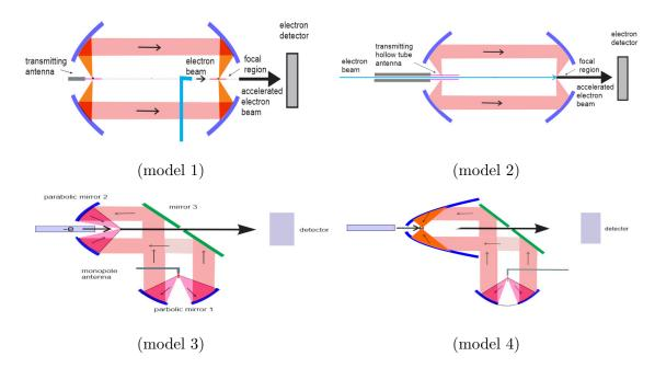
Figure 4.3: different models of two-mirror system accelerator
