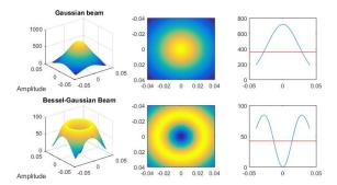
Figure 2.5: Gaussian beam and Bessel-Gaussian beam
