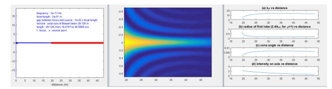
(3) frequency=100 GHz, focal length (fl)=0.19 m, gap= $0.01 \times fl$
