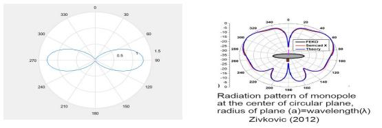
(a) Radiation pattern of monopole without (b) Radiation pattern of monopole with plane
