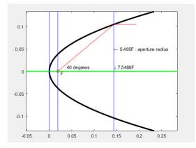
Figure 4.15: Diagram of parabolic mirror for subtending angle 140 degrees
