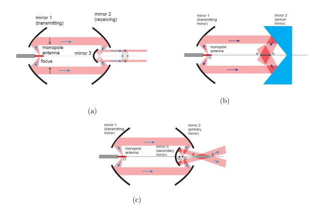
Figure 5.3: Schematics of Bessel beam
