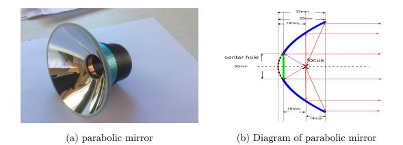
Figure 3.5: Parabolic reflector
