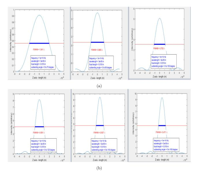
Figure 4.6: different lengths of spot size depending on range of integral angle
