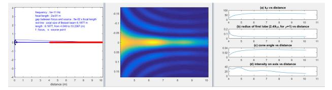
(4) frequency=100 GHz, focal length (fl)=0.19 m, gap=0.05  $\times$  fl
