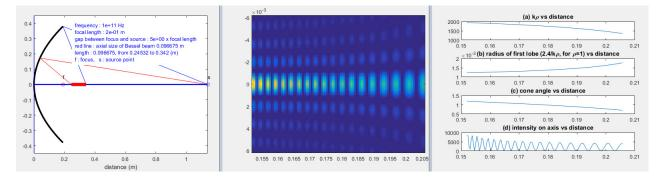
(7) frequency=100 GHz, focal length (fl)=0.19 m, gap= $5 \times \text{fl}$
