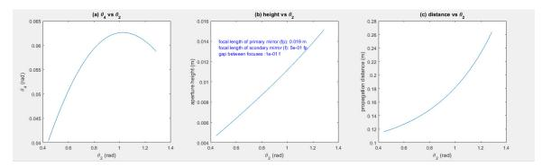
Figure 5.5: relations of cone angle  $(\theta_4)$ , aperture height and propagation distance vs incident beam angle  $(\theta_2)$
