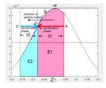
Figure 4.2: mechanism of energy gain
