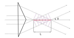
Figure 5.1: Diagram of axicon generating quasi Bessel beam
