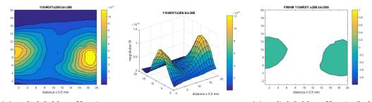
(a) radial field on X axis contour (b) radial field on X axis surf (c) radial field on X axis (half maximum)
