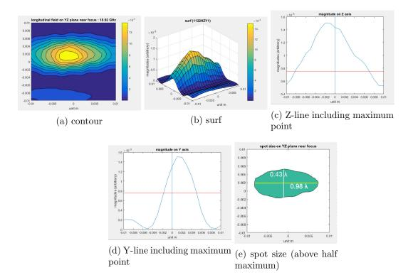
Figure 3.10: longitudinal component on YZ plane
