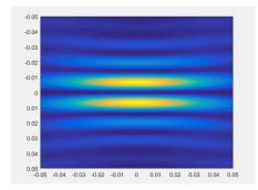
Figure 2.4: Poynting vector in the focal region of radially polarized beam
