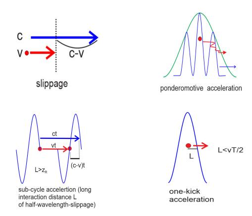
Figure 4.1: different models of vacuum acceleration
