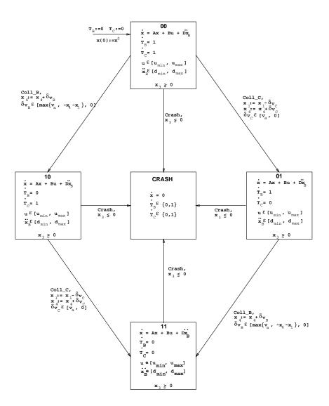
Figure 6: Hybrid Automaton for Automated Vehicle Operation
