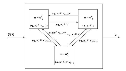
Figure 3: Controller automaton for switching between control objectives
