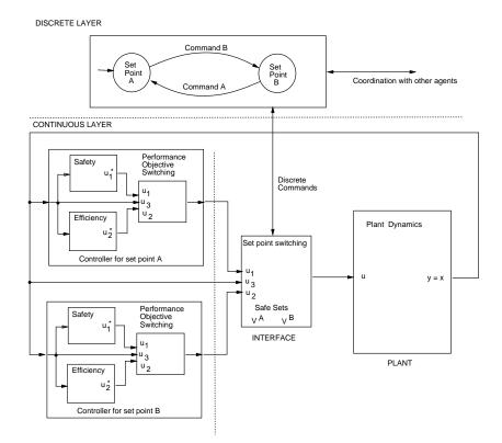
Figure 4: Hybrid controller for a single agent
