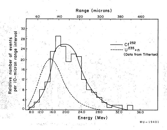
Fig. 2. Energy spectrum of long-range alpha particles associated with fission. Cf<sup>252</sup>, \_\_\_\_\_U<sup>235</sup> + n (Data from Titterton et al.<sup>24</sup>).
