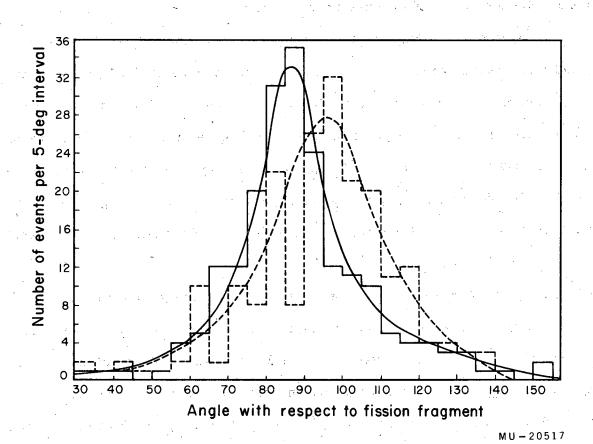
Fig. 3. Number of events per interval vs angle of alpha particle with respect to fission fragment for Cf<sup>252</sup>
