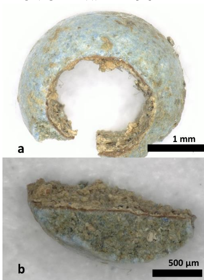
Figure 3-1. a. A digital microscopic image of the overview of a faience bead containing Chinese blue pigment from the Late Warring States Period, Tomb M4, Majiayuan Cemetery, Zhangjiachuan, Tianshui City, Gansu Province, China. b. A cross section through the faience bead, showing a glazed layer that is rich in Chinese blue pigment crystals and a core faience body that is rich in quartz.
