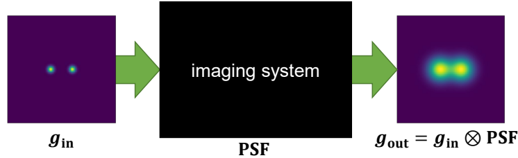
Figure 2.11: A microscope can be described as a linear system with object inputs (like two points, g_{in} ) that are transformed into image outputs by convolution with the microscope point spread function (PSF) that blurs every point in the input plane to a blob when imaged or mapped to the output plane, as in g_{out} .
