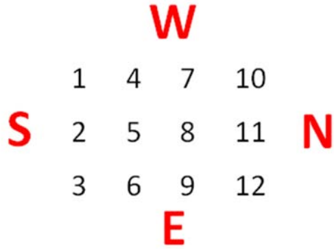
Figure 4.3: Numbering scheme for a 12 point matrix. The numerical values of this matrix would represent a discretized refractive index profile of a waveguide, such as the one shown in Fig. 4.1(a)
