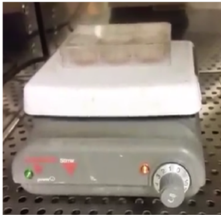
Figure 5.3: A) Schematic of OPCs encapsulated in thermoresponsive gel within spinner flask bioreactor. B) Experimental setup for pilot experiment i. 6 -well dish with hPSCs encapsulated in thermoreversible gel on stirplate. ii. static and stirred 50 RPM wells of 3D hPSC culture in 6-well plate.
