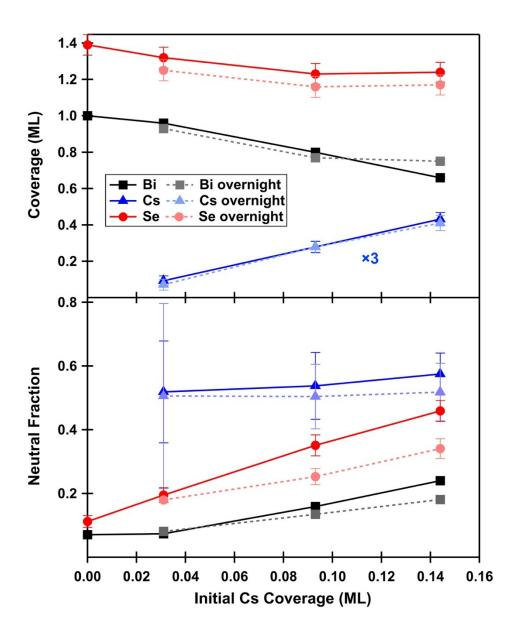
**Figure 4**. Se, Cs and Bi coverages and neutral fractions for 3.0 keV Na<sup>+</sup> singly scattered in single alignment from an IBA-prepared Bi<sub>2</sub>Se<sub>3</sub> sample shown as a function of the initial Cs coverage. The points connected by solid lines were derived from LEIS spectra collected immediately after deposition, while the points connected by dashed lines are from data collected after the samples sat in the UHV chamber overnight (about 9 hrs) at room temperature.
