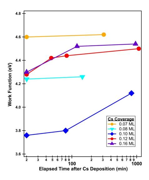
Figure 3. The measured work function with the samples held at room temperature shown as a function of time after various Cs depositions on IBA-prepared  $Bi_2Se_3$ .
