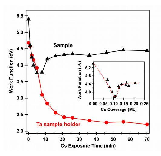
**Figure 1.** Work function of an IBA-prepared  $Bi_2Se_3$  surface (solid triangles) and the Ta sample holder (solid circles) shown as a function of Cs exposure time. The inset is the same work function data, but instead given with respect to Cs coverage (see text). The dashed line illustrates the trend of the work function change as an aid to the eye and is not a fit to the data.
