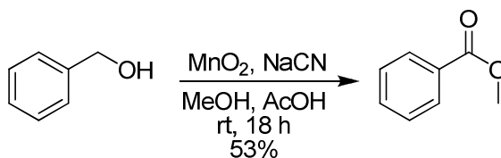
Scheme 2.16: Synthesis of methyl benzoate from benzyl alcohol
