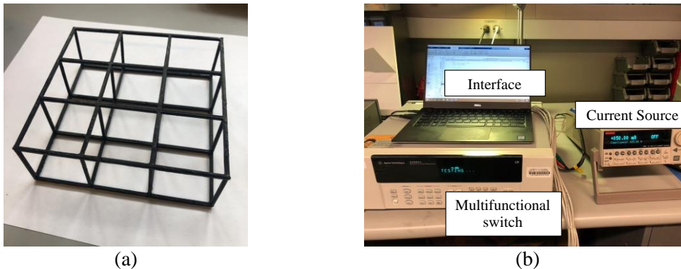
Figure 4.10: (a) A 3 \times 3 \times 1 lattice structure was spray-coated with a conductive, nanocomposite thin film. (b) ERT measurements were obtained using a customized data acquisition system.
