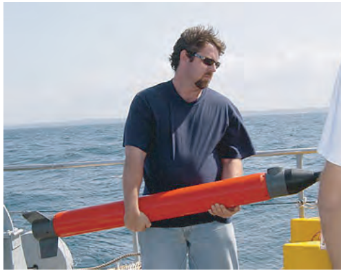
Single Channel Overhauser Scalar Magnetometer UW Tow Configuration Marine Magnetics SeaSPY
