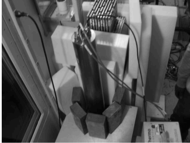
Figure 31. Set up used during the irradiation in air. Polyethylene was used as moderator and some blocks of lead served as neutron reflectors around the generator.
