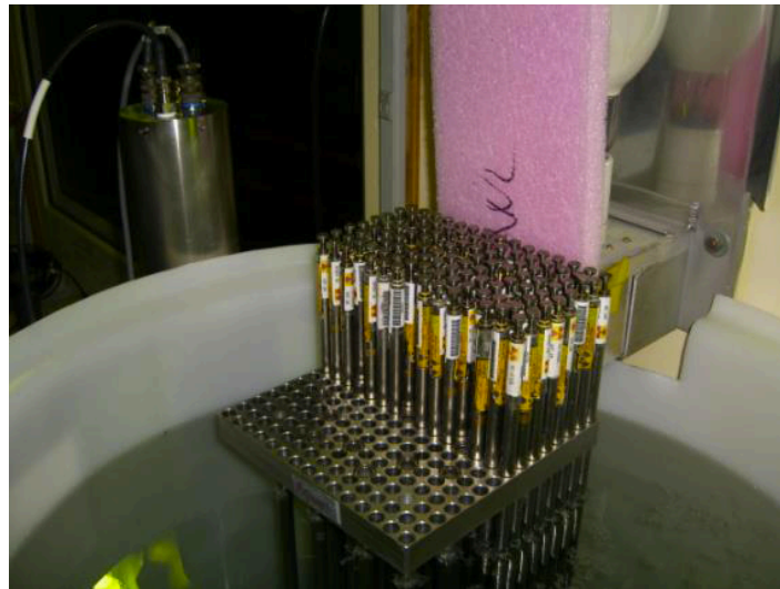
Figure 30: Half-filled assembly rack for “in-water” measurement.
