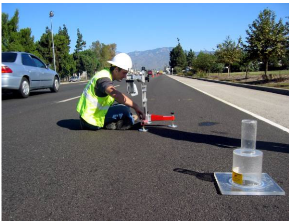
Permeability and Pendulum skid testing
