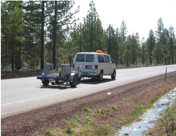
Site selection based on pavement structure (FWD)
