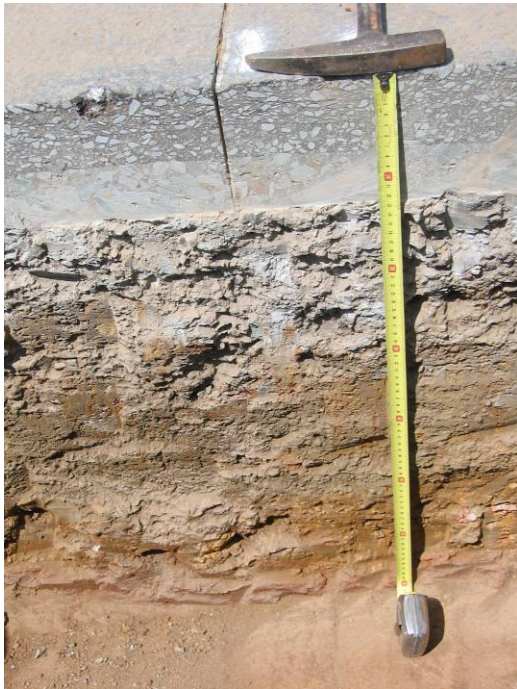
Hand-finished test pit face
