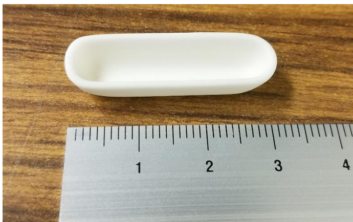
Figure 3.6: Alumina combustion boat from Coorstek 3x1 cm.
