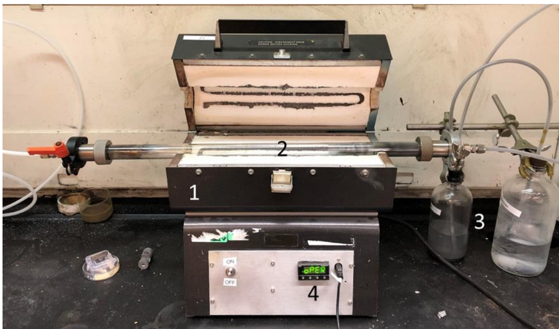
Figure 3.5: Image of a chemical vapor deposition system consisting of a 1) tube furnace 2) quartz reaction tube 3) exhaust bubbler and 4) temperature controller
