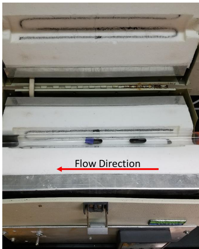
Figure 3.7: MoTe 2 growth set up with molybdenum oxide boat at the center of the furnace and the tellurium boat positioned up stream of the flow to reach max volatility when the furnace is at the maximum hold temperature
