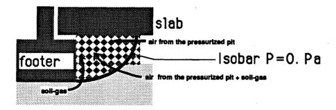
The third factor, a high soil permeability, reduces diffusive entry of radon into the subslab aggregate layer. When the soil is highly permeable, air flows from the subslab aggregate layer into the soil at large enough velocities that diffusion of radon upstream into the aggregate becomes impossible. However, when the soil has low permeability, air velocities from the aggregate into the soil are extremely small, and diffusion of radon
