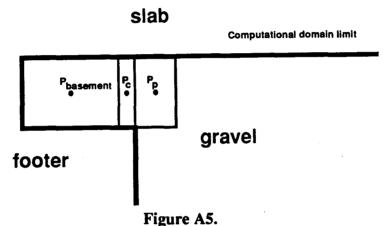
Vertical cross section of the slab-footer crack as modeled by a control volume.
