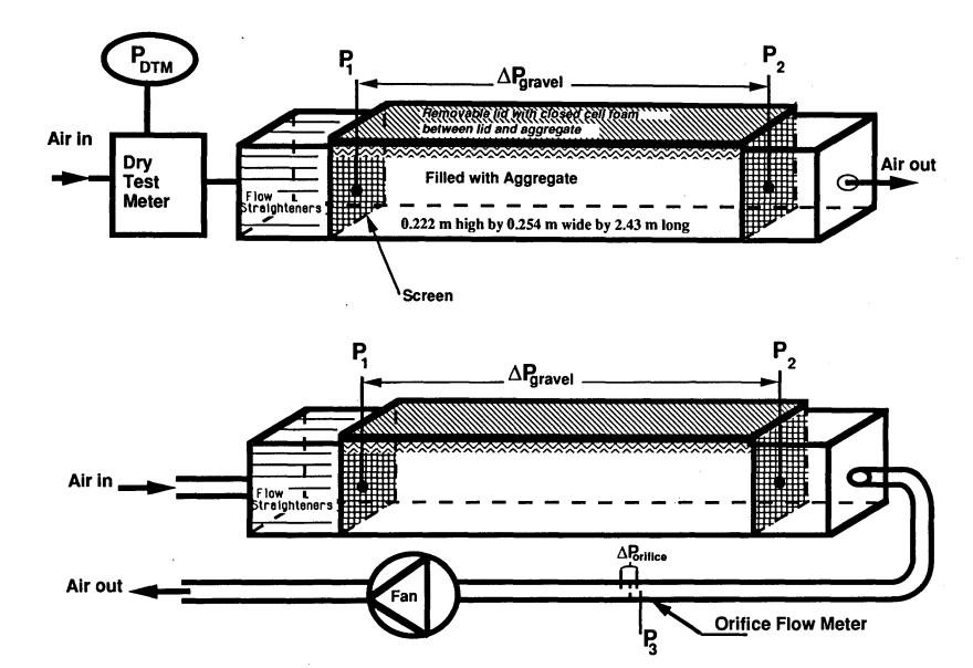
Figure B1. Schematic diagrams of the test apparatus. Low/mid and high/peak velocity data were collected using dry test meters and orifice plate flow meters, respectively, to measure flow rate.
