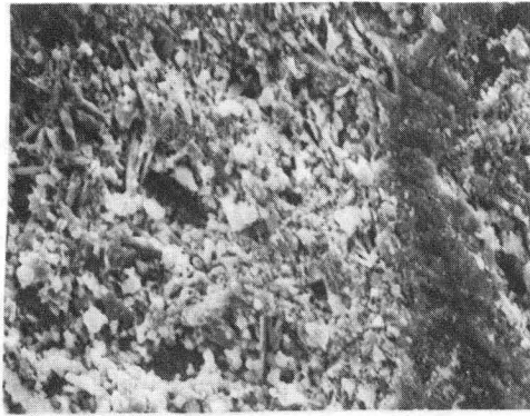
Surface of TiC-Mo washer Temperature=730°C Contact pressure=0.17MPa
