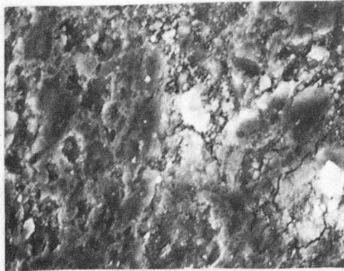
Surface of SCA from TiC-Mo washer test Temperature=25°C Contact pressure=0.69MPa
