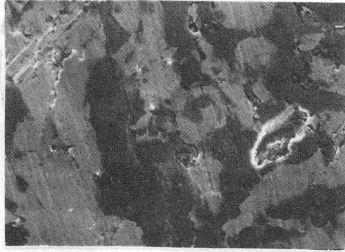
Surface of untested \text{Cr}_3\text{C}_2 -Mo washer 10 \mu\text{m}
