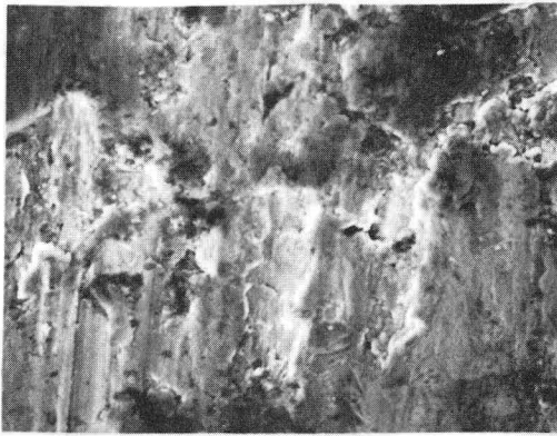
Surface of WC-Mo washer Temperature=425°C Contact pressure=0.17MPa
