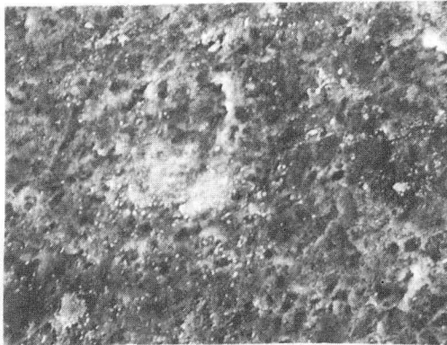
Surface of SCA disc from WC-Mo washer test 10 \mu m Temperature=730°C Contact pressure=0.17MPa
