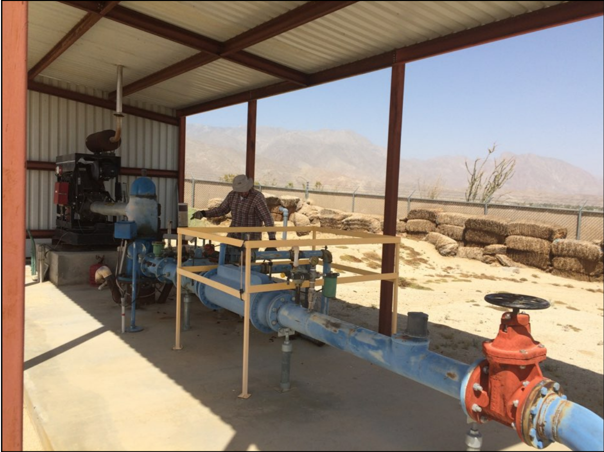
Illustration 2.1: A Department of Water Resources field geologist measures the water levels at a monitoring well in Smoketree. Twice every year, a DWR team takes measurements at wells across Smoketree Valley to chart changes over time.
