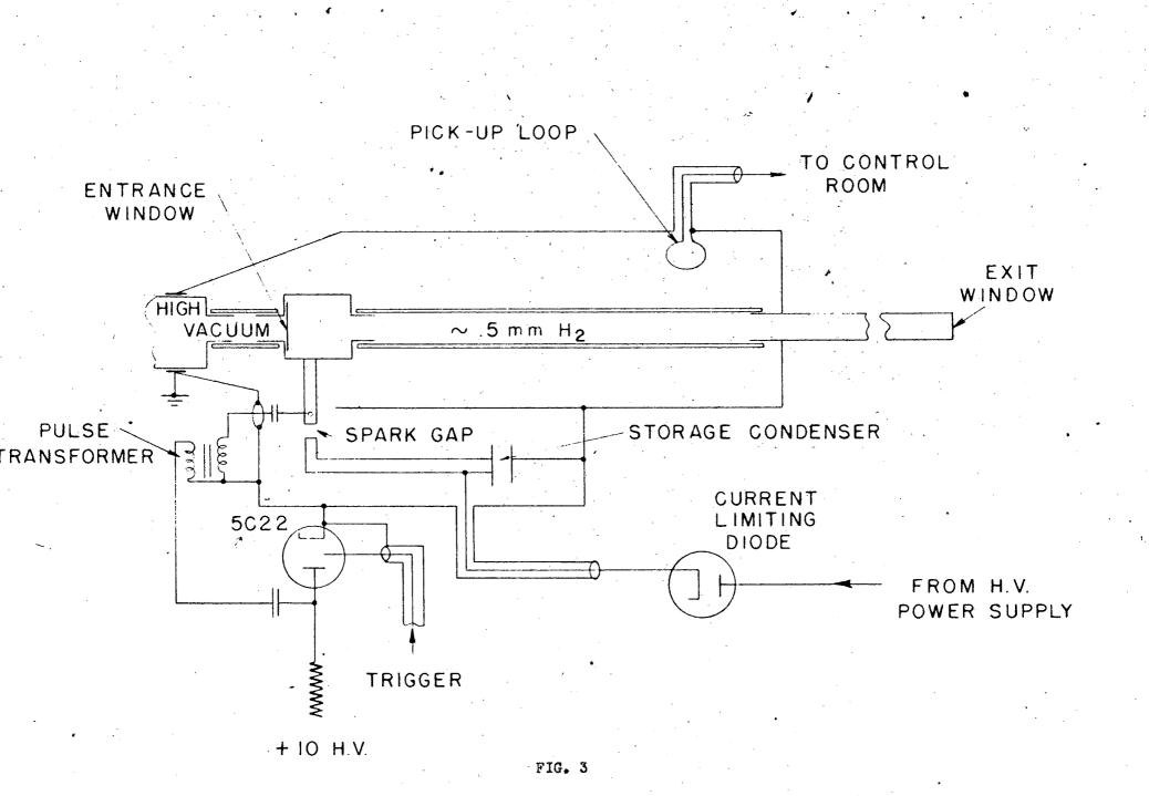
Diagram of arc lens pulse connections. Note the co-axial connections of the storage condenser in relation to the spark gap and discharge tube.
