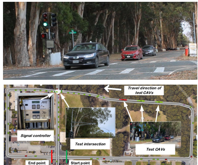
Figure 1. Top: Test CAVs operating on physical test track. Bottom: Layout of the test track.
