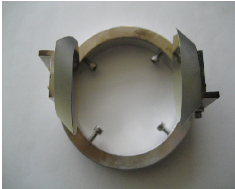
Figure 2.5: Mirrors for the axial flow speed which are mounted on the wall of the side port.
