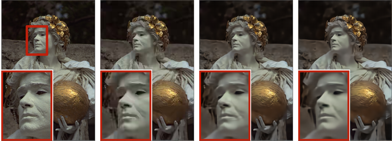
(a) Original image (from Kodak [1993] dataset) (b) BPG 4:4:4; 0.14 BPP (PSNR = 30.4) (c) Proposed (SGA); 0.13 BPP (PSNR = 31.2) (d) [Minnen et al., 2018]; 0.12 BPP (PSNR = 29.8)
