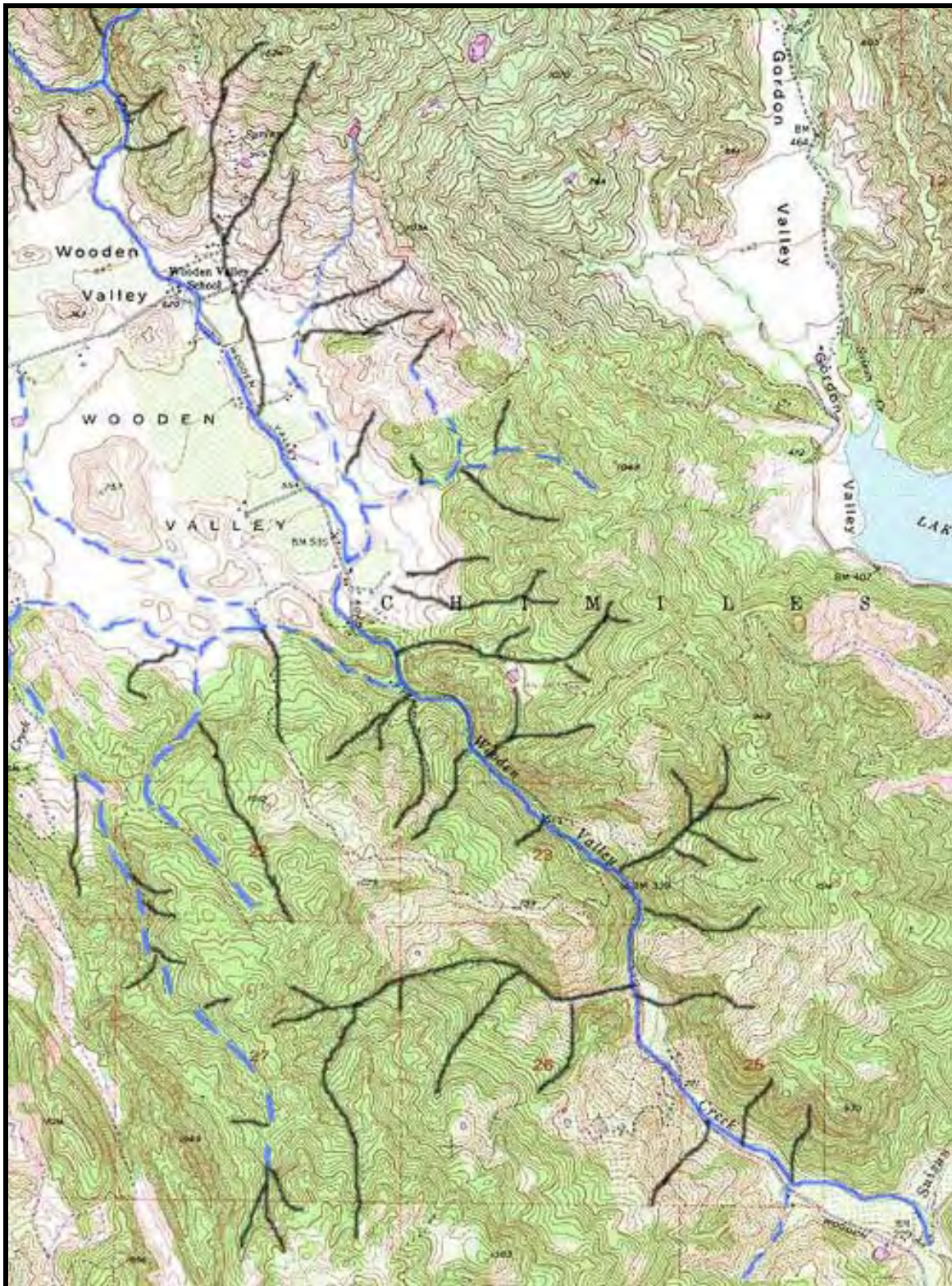
Figure 14. A Portion of Wooden Valley Creek Subbasin Illustrating Year-Round and Seasonal Creeks in Blue and Ephemeral Creeks in Black
