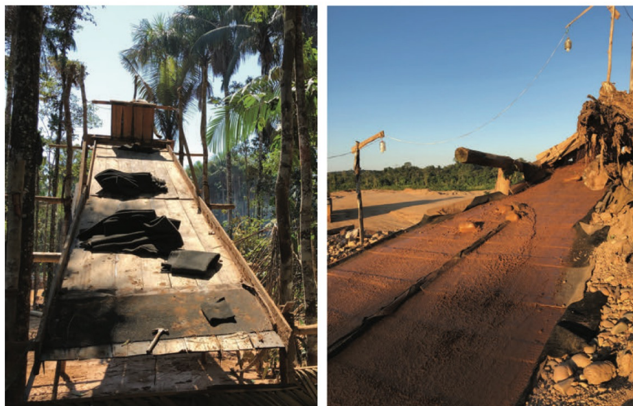
Figure 2. Sluices constructed on-site in a traca based operation (left) and a heavy machinery-based operation in Madre de Dios, Peru. Sluices are lined with carpets to capture fine gold particles present within alluvial sediments and soils. Note that the number of carpets differs between these operations as greater volumes of gold-bearing material are processed in heavy machinery-based operations.
