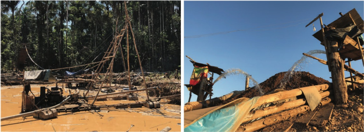
Figure 1. Diverse modalities of gold production in the small-scale gold mining economy in Madre de Dios, Peru. Left, the traca , a dredge set floating on a raft supported by empty oil drums that works by suctioning slurries of gold-bearing soils from the bottom of an open pit mine. Right, huaychuleros , sit atop wooden cabins in a heavy machinery-based production modality. The huaychuleros are responsible for washing gold-bearing soils deposited at the top of the sluice by a dump truck.
