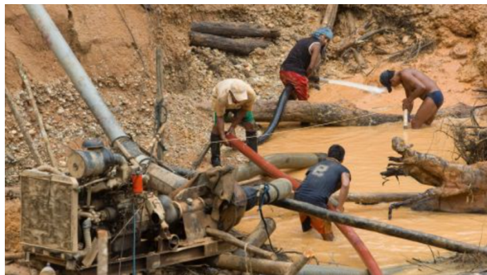
Figure 5. The chupadera is a production modality featuring two large motors that are used in tandem to power high-pressure hoses and suction gold-bearing slurries to a sluice box.
