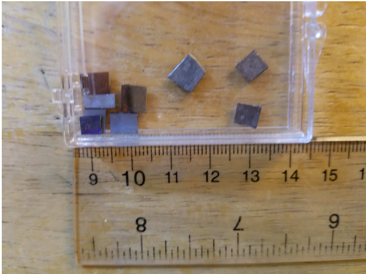
Figure 26 Image of diced silicon samples of varying sizes from \sim 0.25 to \sim 0.5 \text{cm}^2 .
