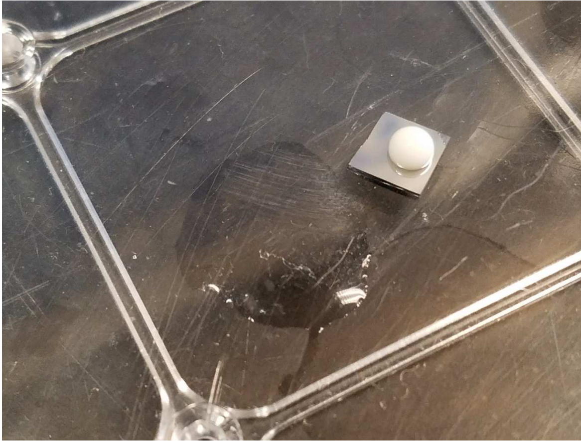
Figure 27 Image of slurry drop on top of Si substrate.
