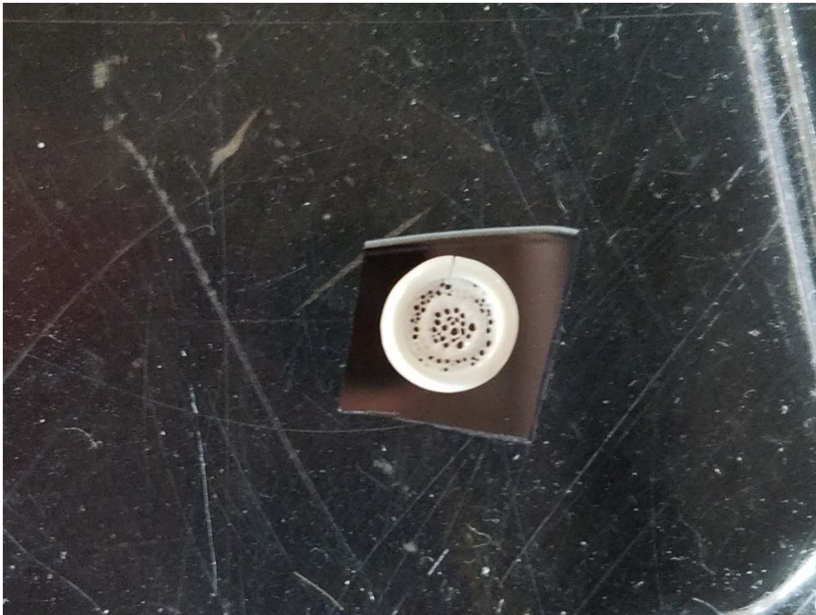
Figure 28 Image of slurry dropped after it has been dried.
