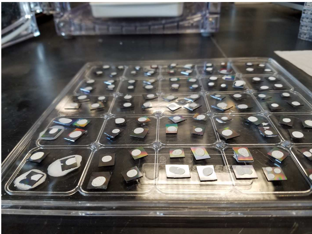
Figure 37 Dried samples of HAp on Si, ready for scraping and sintering.
