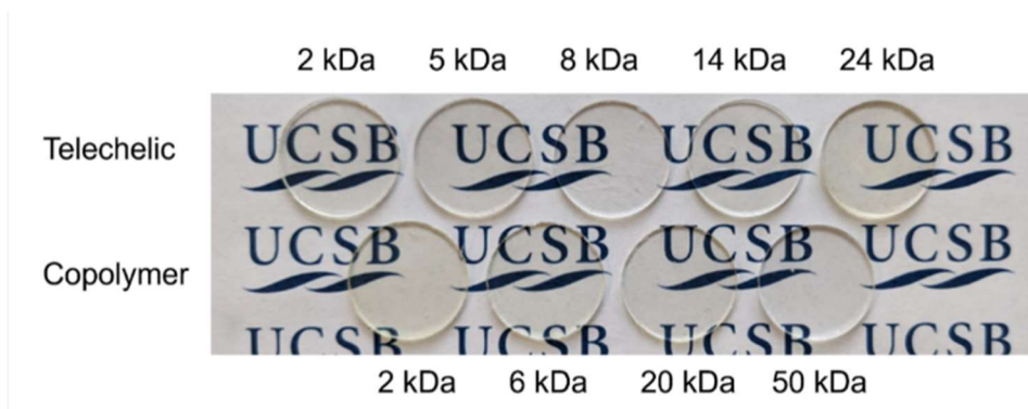
Figure 3.9. Representative image of rheology discs made from the listed starting polymer and tris(dimethylvinylsilyl) borate. Yellow tinge is due to Pt clusters precipitating from Karstedt's catalyst during curing.
