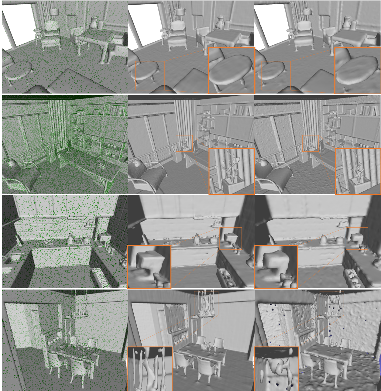
Figure C.2: Left: Ground truth mesh overlaid with input point samples; Middle: Our reconstruction; Right: Screened PSR [55] reconstruction. The input are point samples from the SceneNet ground truth mesh at a sample density of 500 \text{ points} / m^2 .
