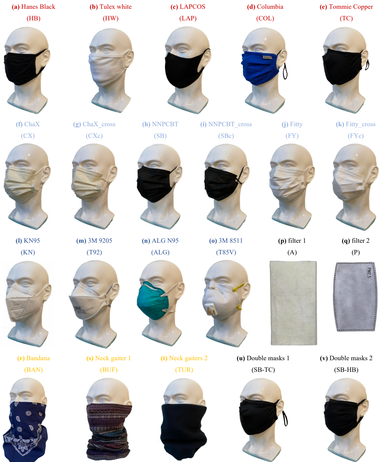
Figure 1. Images of the face coverings used for the experiments. Fig.1 is an illustration of a real person wearing face covering. We investigated four types of face covering and various wearing styles, including (a)-(e) cloth masks, (f)-(k) surgical masks in regular and cross ear loop style, (l)-(o) KN95 and N95 respirators, (r)-(t) bandana and neck gaiters, (u)-(v) double masks with a cloth mask outside and a surgical mask inside. (p) and (q) are two types of masks filters, which can be inserted to the inner layer of the masks.
