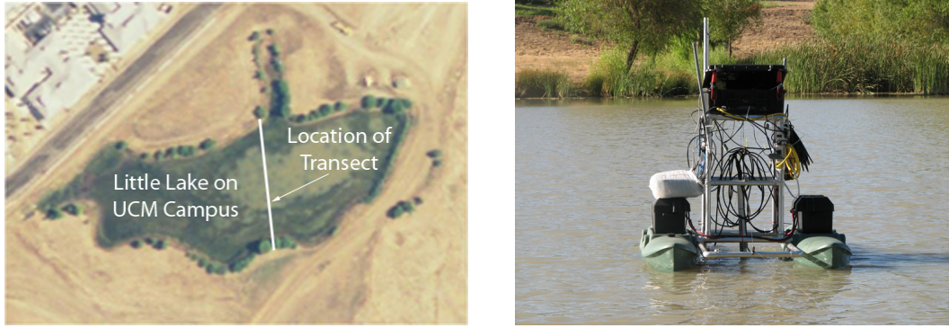
Figure 5.2: Satellite map of the UC Merced campus lake with experimental transect labeled and NIMS AQ operating on the lake with the sonar and other sensors attached
