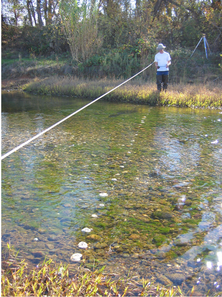
Figure 8. Placement of 1 st set of tracer gravel lines at Bear River site, BR2. A second set of stone was placed approximately 0.5m upstream soon after the photo was taken. Note the relatively undisturbed bed and low-elevation of the stationing tape, which allowed for precise relocation in the event of aggradation.
