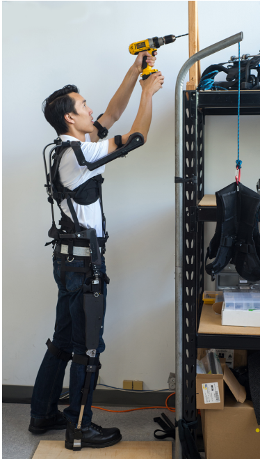
Figure 113. General load transfer during overhead work with shoulder-leg system.
