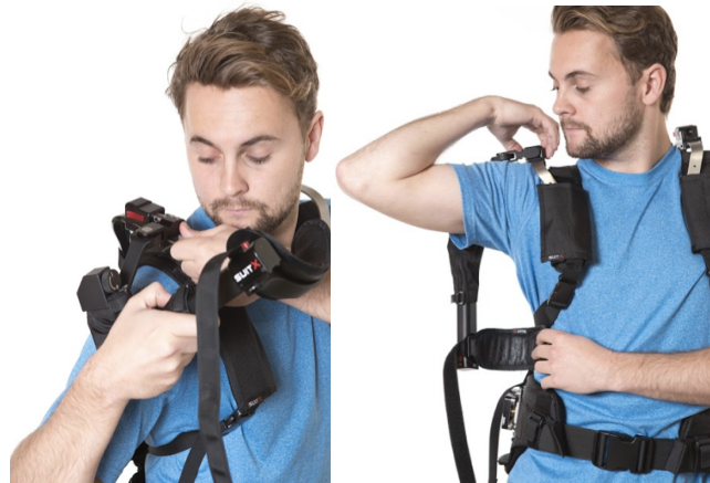
Figure 58. Donning of the arm unit (a) aligning & inserting (b) checking/releasing.
