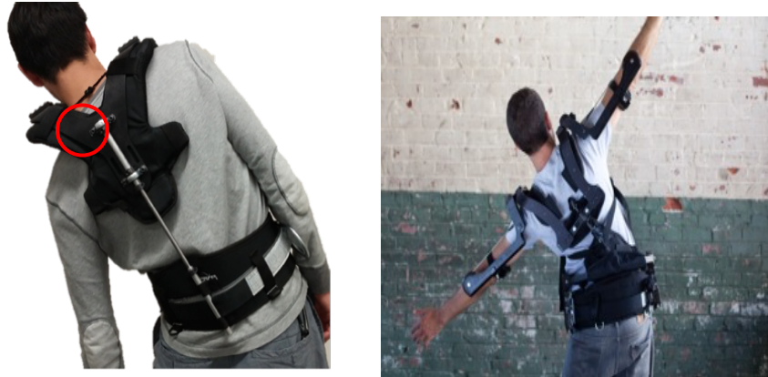
Figure 80. Effects of lateral spinal flexion joint vertical location (a) Va (b) V0.
