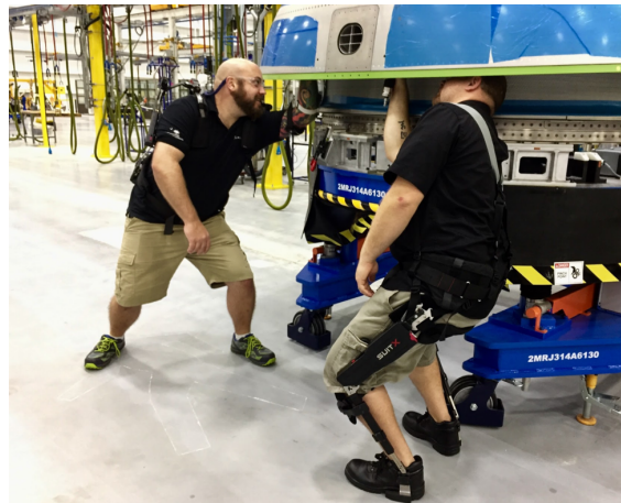
Figure 111. Low Ceiling Work with shoulder-leg system.
