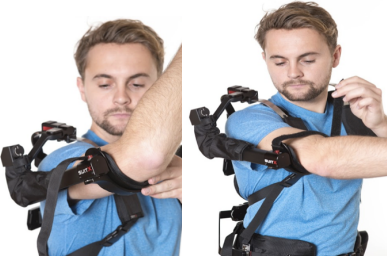
Figure 43. Donning the arm coupler (a) arm cuff and (b) arm strap.
