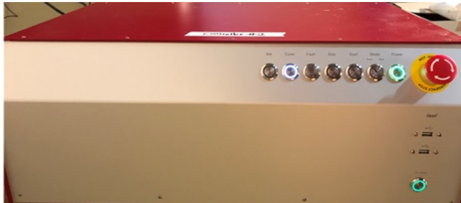
Figure A.7: Linear Stage Controller Front Panel (1 of 2 controllers depicted)
