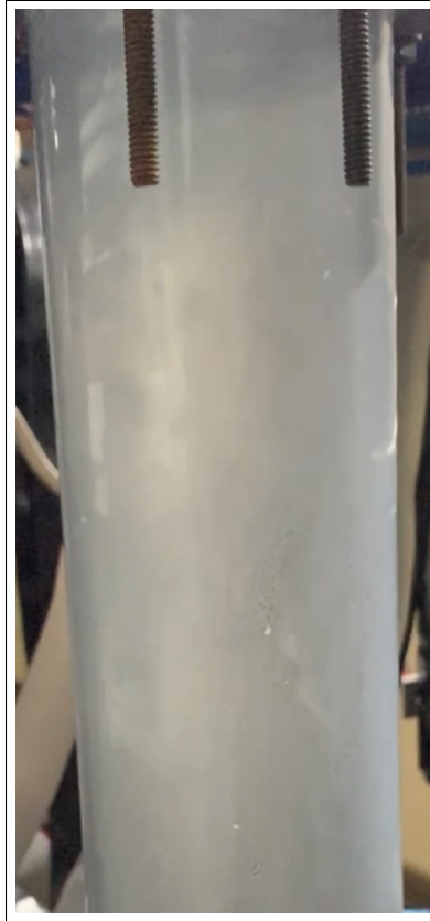
Figure 9.32: Picture of Opaque Bubble Column - Inner Wall coated with Superhydrophobic Coating (NeverWet)
