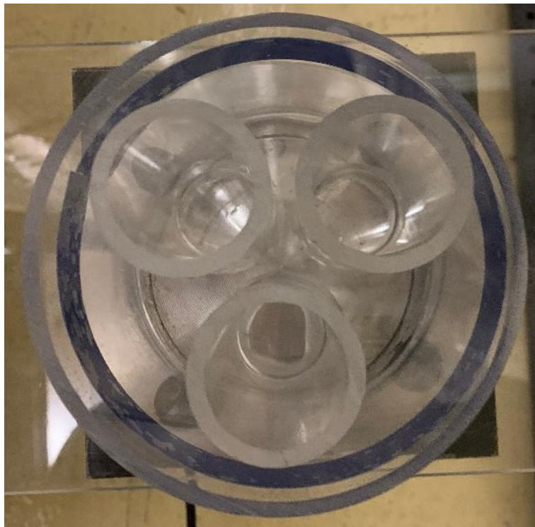
Figure B.11: Three-Dimensional Image of Acrylic Cylinder with Three Acrylic Inner Tubes
