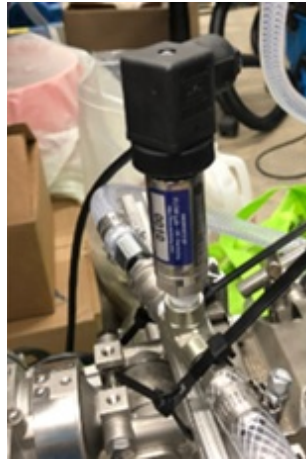
Figure 5.4: UNIK5000 - Absolute Pressure Transducer
