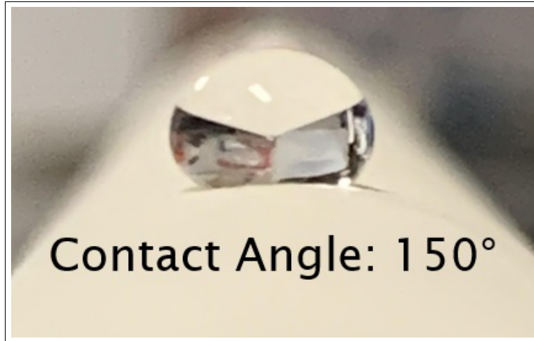
Figure 10.16: Single Bubble on SHS-coated PVC Tube with Contact Angle measured by ImageJ imaging software.
