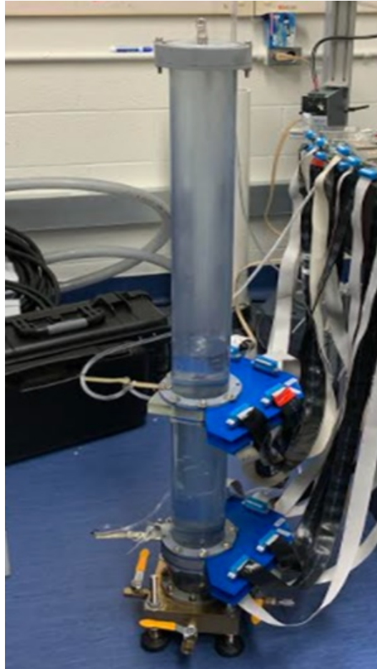
Figure 7.3: Bubble Column with four wire mesh sensors
