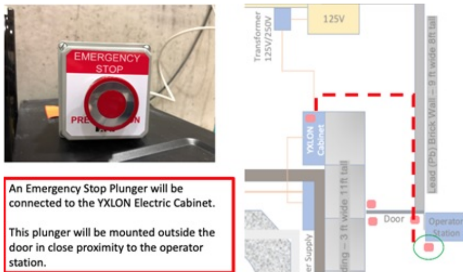
Figure A.15: YXLON X-ray Emergency Stop Plunger
