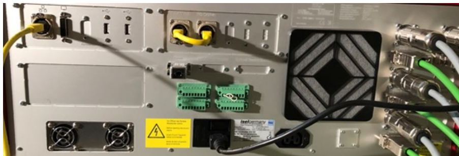
Figure A.8: Linear Stage Controller Back Panel (1 of 2 controllers depicted)
