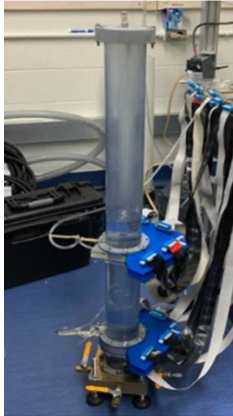
Figure 9.3: Bubble column with four Wire Mesh Sensors installed
