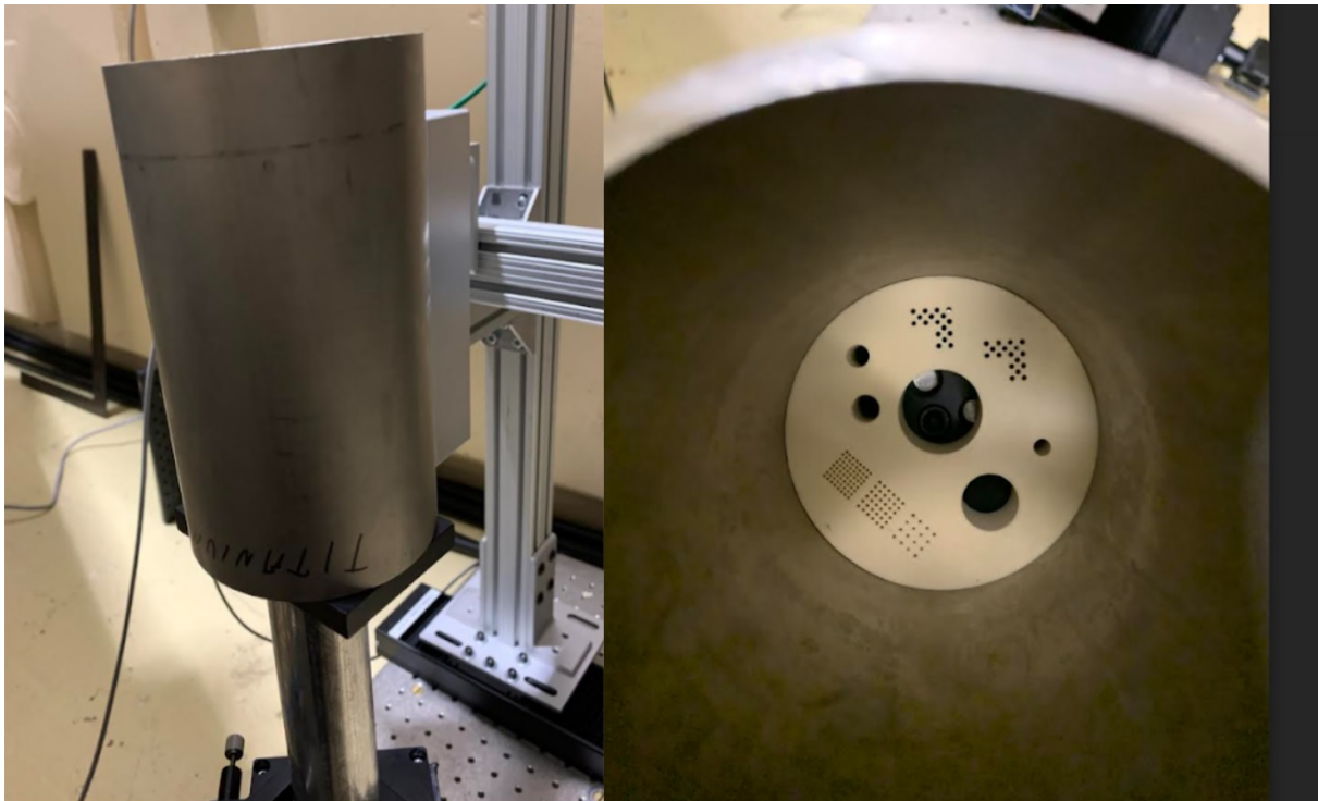
Figure 8.42: Bubble phantom inside titanium pipe (left: sideview; right: topview)
