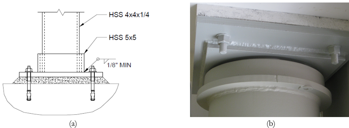
Figure 10. Detailing to avoid composite action using (a) telescoping HSS and (b) isolator
