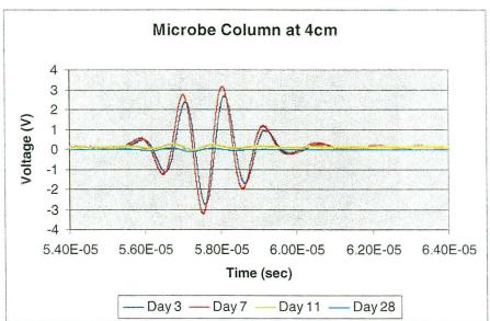
Figures 3.6 and 3.7: Acoustic waveform data from the microbe inoculated column for the 8cm and 4cm depth locations over four periods of time. Note the travel time differences and amplitude decreases as a function of time and gas evolution.
