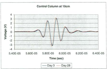
Figures 3.8 and 3.9: Acoustic waveform data from the control column for the 12cm and 10cm depth locations over two periods of time. Note the high degree of repeatability of the waveforms. Such repeatability suggests that the effects observed in the inoculated column are exclusively biogenic in origin as the control column received the same saturating medium.
