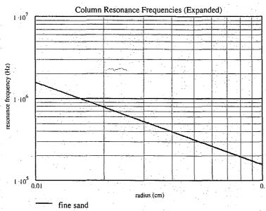
Figures 4.1: Mathematical estimation of the resonance frequencies corresponding to a wide range of bubble sizes (lower image is an expanded view). The parameters used here match those believed to exist within the columns.
