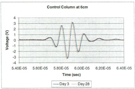
Figures 3.10 and 3.11: Acoustic waveform data from the control column for the 8cm and 6cm depth locations over two periods of time. Note the high degree of repeatability of the waveforms.
