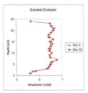
Figures 3.17: Graph of changing wave amplitudes over the experiment for both the microbe-inoculated and the control column. Note the lower values both high and low in the control column which are likely due to initially entrapped air during saturation. There is no observed temporal change, however.
