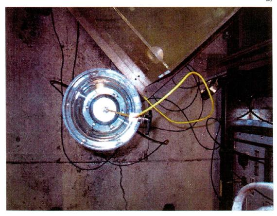
Figure 2.6: Photograph showing the apparatus designed to make acoustic wave measurements from the top. The 180° alignment of the transducers is visible as is their offset from the column wall.
