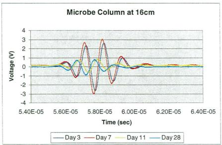
Figures 3.4 and 3.5: Acoustic waveform data from the microbe inoculated column for the 24cm and 16cm depth locations over four periods of time. Note the travel time differences and amplitude decreases as a function of time and gas evolution.
