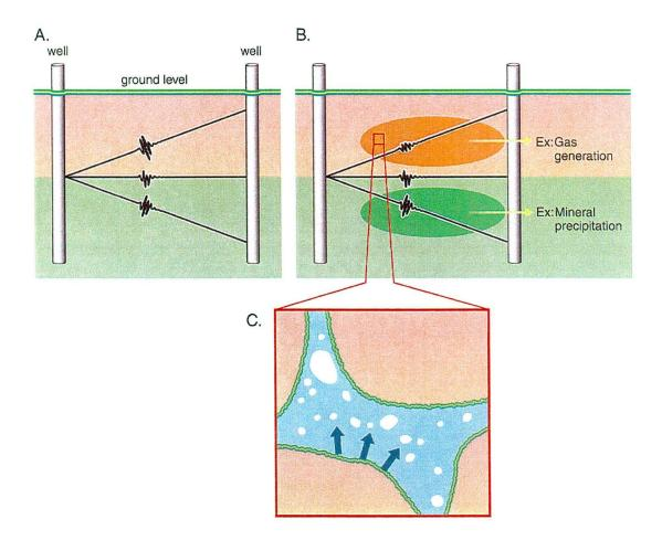
Figure 1.2: Illustration showing the potential layout of a cross-well geophysical system designed to monitor terrestrial subsurface microbial activity over time. Only a few of the many potential acoustic wave paths are shown. Note that changes in subsurface conditions may arise through a variety of means, not solely gas production. Attenuation of acoustic wave energy through a region of gas production is shown in b) for the conditions depicted in c).
