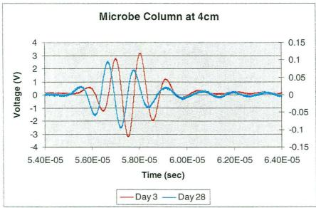
Figures 3.14 and 3.15: Acoustic waveform data from the inoculated column for the 8cm and 4cm depth locations over two periods of time. The voltage scale for the attenuated signal (Day 28) is shown on the right. Note the differences in travel times.
