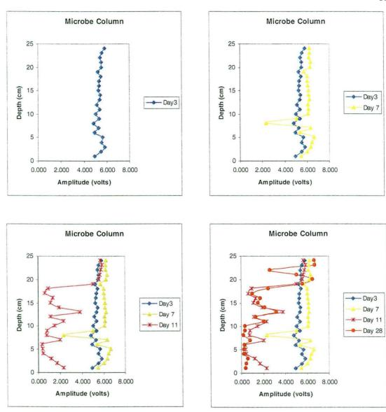
Figures 3.16: Series of graphs illustrating change in the measured wave amplitudes over the four periods shown in Figures 3.4 to 3.7. The onset of gas at the 8cm location is followed by abrupt gas production throughout the column shortly thereafter. Note the lack of attenuation of those waves transmitted through the uppermost portion of the column.
