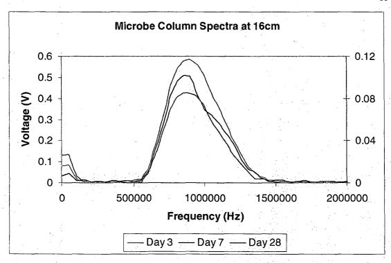
Figures 3.19: Inoculated column waveform spectra for the 16cm location over three time periods (Day 28 voltage scale is on the right). Note the selective attenuation of frequencies above 950kHz. These correspond to damping losses associated with very small diameter bubbles or more likely, scattering off of larger diameter bubbles.
