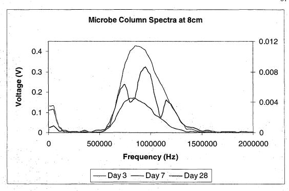
Figures 3.20: Inoculated column waveform spectra for the 8cm location over three time periods (Day 28 voltage scale is on the right). Note the selective attenuation of frequencies between 750 and 950kHz and above 1MHz. These may correspond to both damping losses associated with a range of pore-filling bubble sizes and to wave scattering.
