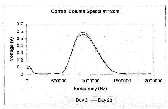
Figures 3.21: Control column waveform spectra for the 12cm location over two time periods. Note the high degree of repeatability in the two spectra over the course of nearly one month.
