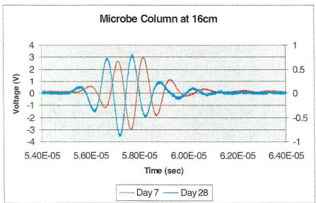
Figures 3.12 and 3.13: Acoustic waveform data from the inoculated column for the 24cm and 16cm depth locations over two periods of time. The voltage scale for the attenuated signal (Day 28) is shown on the right. Note the differences in wave travel time.
