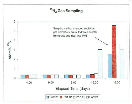
Figure 3.3: The results of the isotope ratio mass spectrometer analysis of evolved column  $^{15}\mathrm{N}.$  The gas sampled over the first two weeks of the experiment shows no deviation from atmospheric atom%  $^{15}\mathrm{N}$  (0.3663) but breakthrough of labeled gas appears to transpire once pressure within the column rises enough to enhance diffusion into the samplers. The final results indicate that respired  $\mathrm{N}_2$  was the only reasonable source of gas within the columns.
