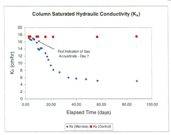
Figure 3.1: The results of the saturated hydraulic conductivity  $(K_{\rm s})$  measurements over the course of the experiment. The first indication of gas within the acoustic monitoring column is show for comparison. Note that very little decrease in  $K_{\rm s}$  occurs before this time but that the values drop rapidly once gas appears, ultimately stabilizing to a final value. The results from the control column are also shown for comparison.
