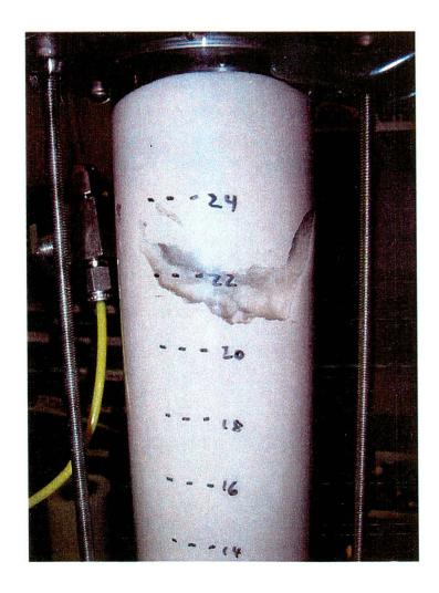
Figure 3.2: Close-up photograph of the acoustic monitoring column after 60 days have elapsed since saturation. The bubble accumulation observed in this column was similar to that observed in the other inoculated columns. Its dimensions were approximately  $2 \, \mathrm{cm} \times 3 \, \mathrm{cm} \times 1 \, \mathrm{cm}$  and it possibly represents entrapment and accumulation along a packing discontinuity.
