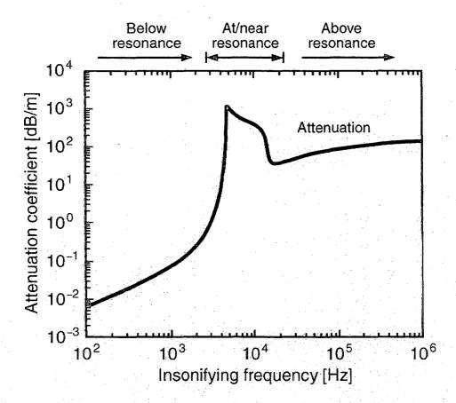
Figures 4.2: Modeled prediction of wave attenuation coefficients in fine sand for a wide range of frequencies (modified from Tuffin et al., 2000). Note that the conditions modeled here are not an exact analog for those in the columns. Rather the figure is included to illustrate the dramatic increase in attenuation possible when transmitting frequencies closely match the particular resonance frequency of bubbles in the sediment.
