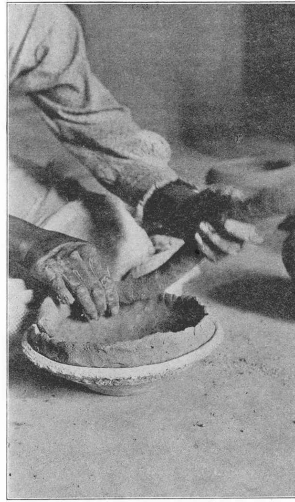
a Applying the first roll of clay to the base. The roll is held in the left hand, and is flattened and pinched into place in the inside of the rim by the fingers of the right hand.
