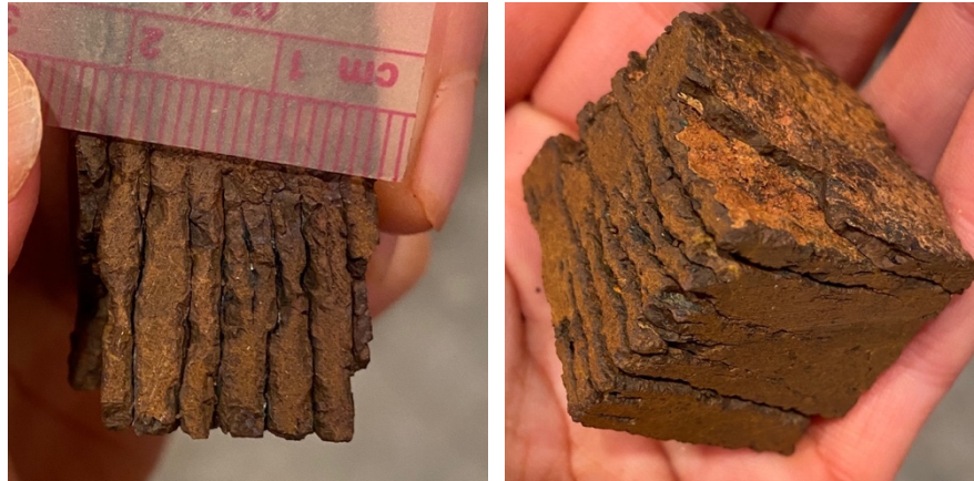
Figure 4.3: Two pieces of one of the mudstone rocks from Feature 5, post-cutting. Note the orange-brown hue to the rocks. This color is seen in all the mudstones but reverts to a bright red-brown hue upon laboratory heating in air. The silty-mud layers vary in thickness from roughly 2-3mm (left image) but in some areas are completely conjoined (right image). The rock preferentially breaks along the voids between the silty-mud layers and is most stable in areas where the layers have conjoined.
